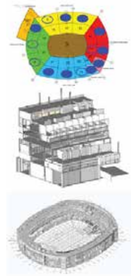
WBS - Work Breakdown Structure Above is an example of the WBS employed at the Meadowslands, where the project was broken into 27 distinct areas. 3D MEP coordination followed this format, by floor.
